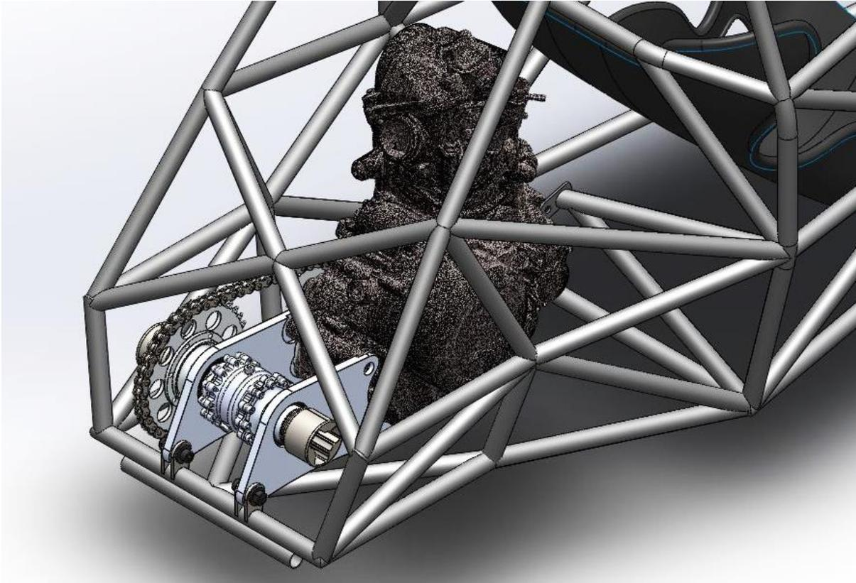
**Figure 5:** 3D CAD model isometric view of the UA-20 concept highlighting internally mounted drivetrain assembly with differential hangers mounting to rear of engine.
