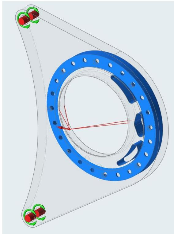
**Figure B1:** Blue highlighted region signifies a rigidly bonded connection between two parts.
