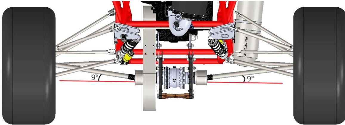
**Figure 3:** 3D CAD model top view of the UA-19 drivetrain showing the extreme driveshaft angles.
