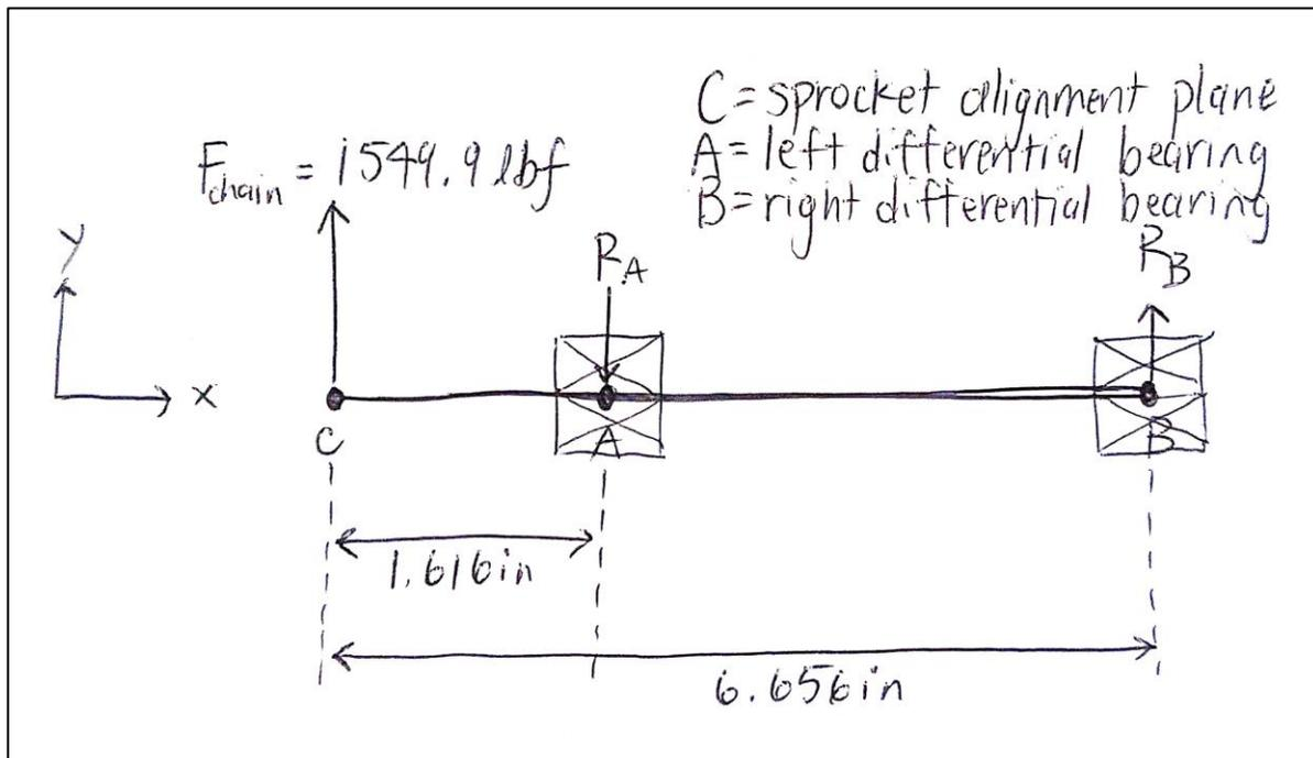
**Figure F1:** Differential bearing reaction forces.
