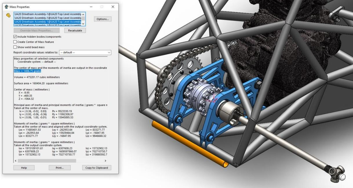
**Figure 15:** Mass analysis done in SolidWorks displaying drivetrain mounting system to be 1406.75 g.
