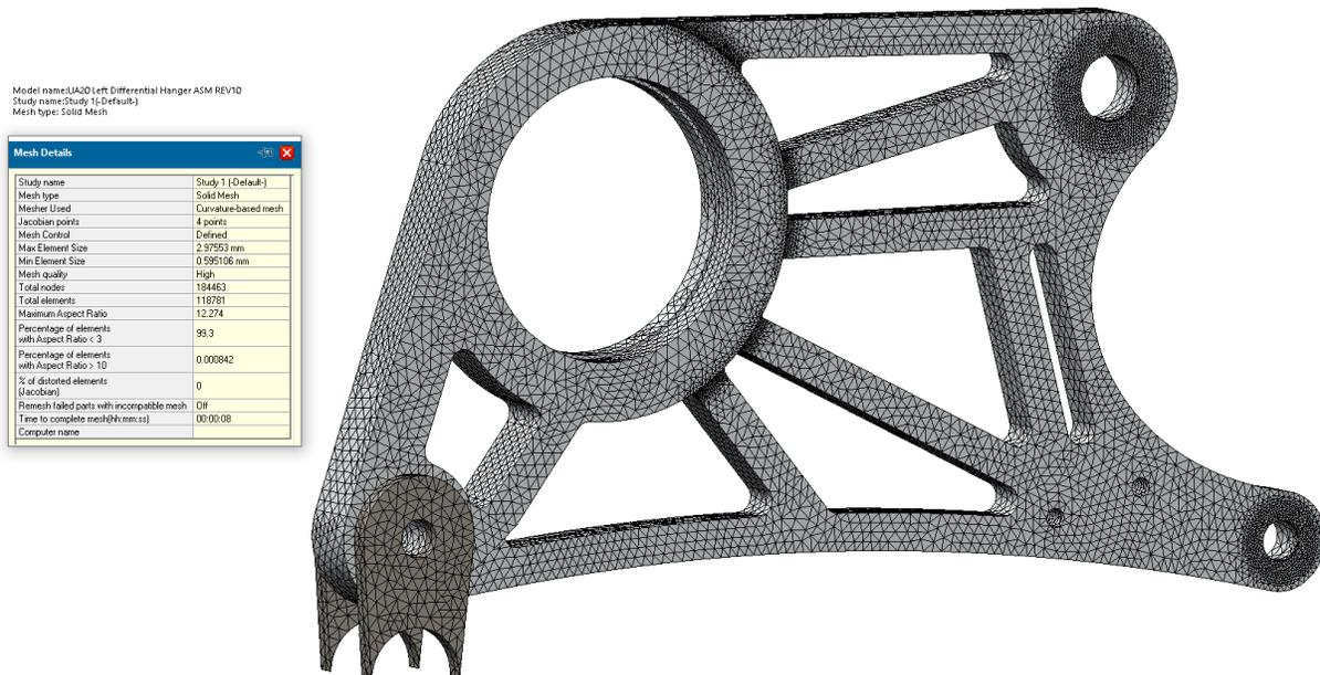
**Figure E22:** Mesh with maximum global element size of 2.97 mm and mesh control maximum element size of 0.8 mm.
