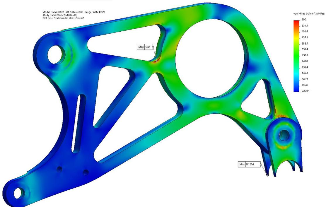
**Figure E16:** vonMises results for iteration 1 – view #2.
