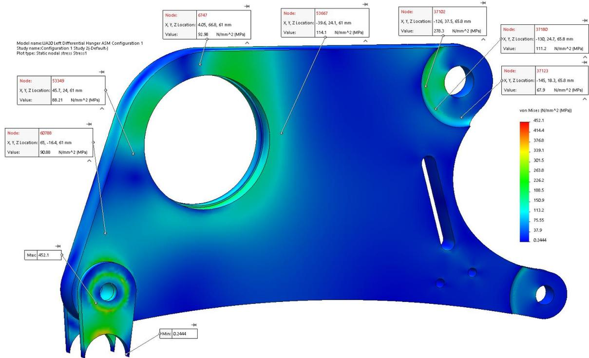
**Figure E13:** von Mises results for mesh 2 with probed sensor locations shown.
