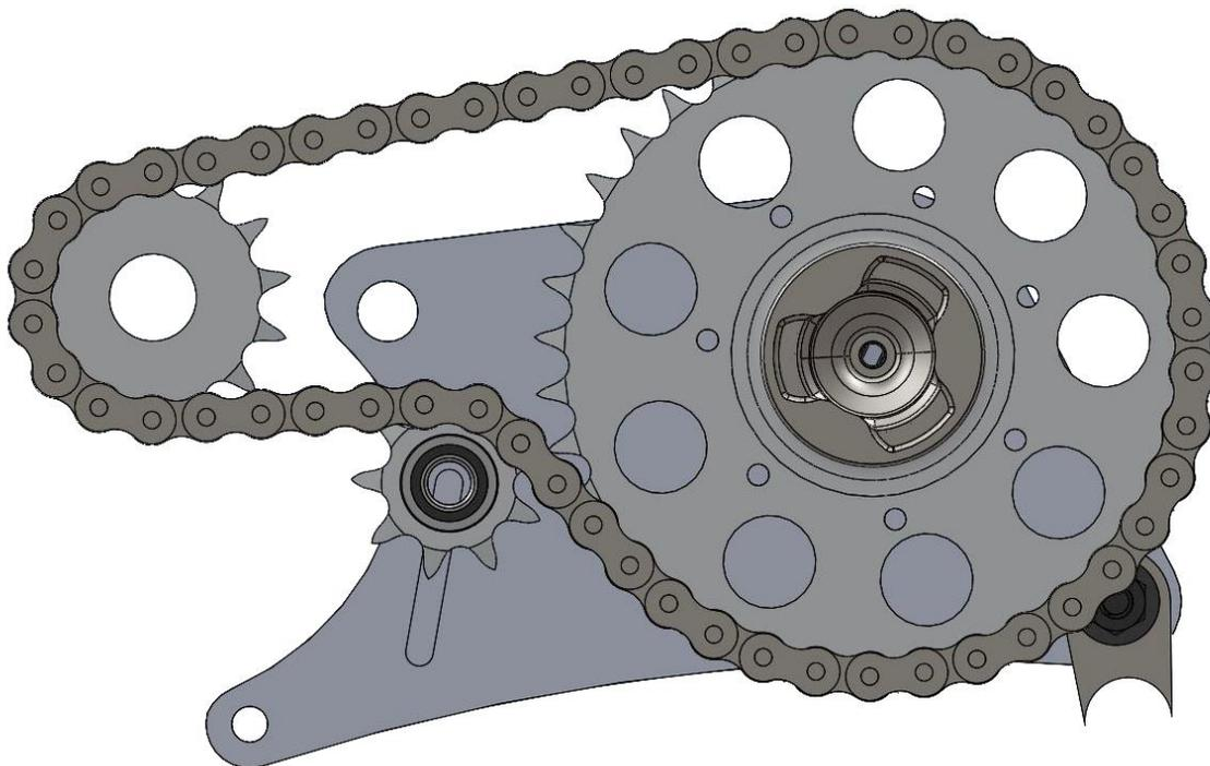
**Figure 7:** 3D CAD model side view of the UA-20 drivetrain assembly highlighting idler sprocket in adjustable slot.
