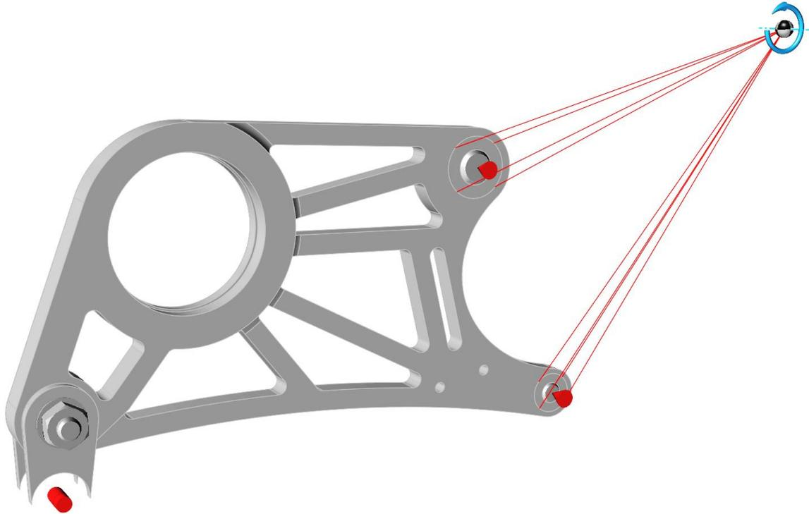
**Figure E29:** 2 g longitudinal engine mass acceleration applied to the differential hanger in Altair Inspire 2019.3
