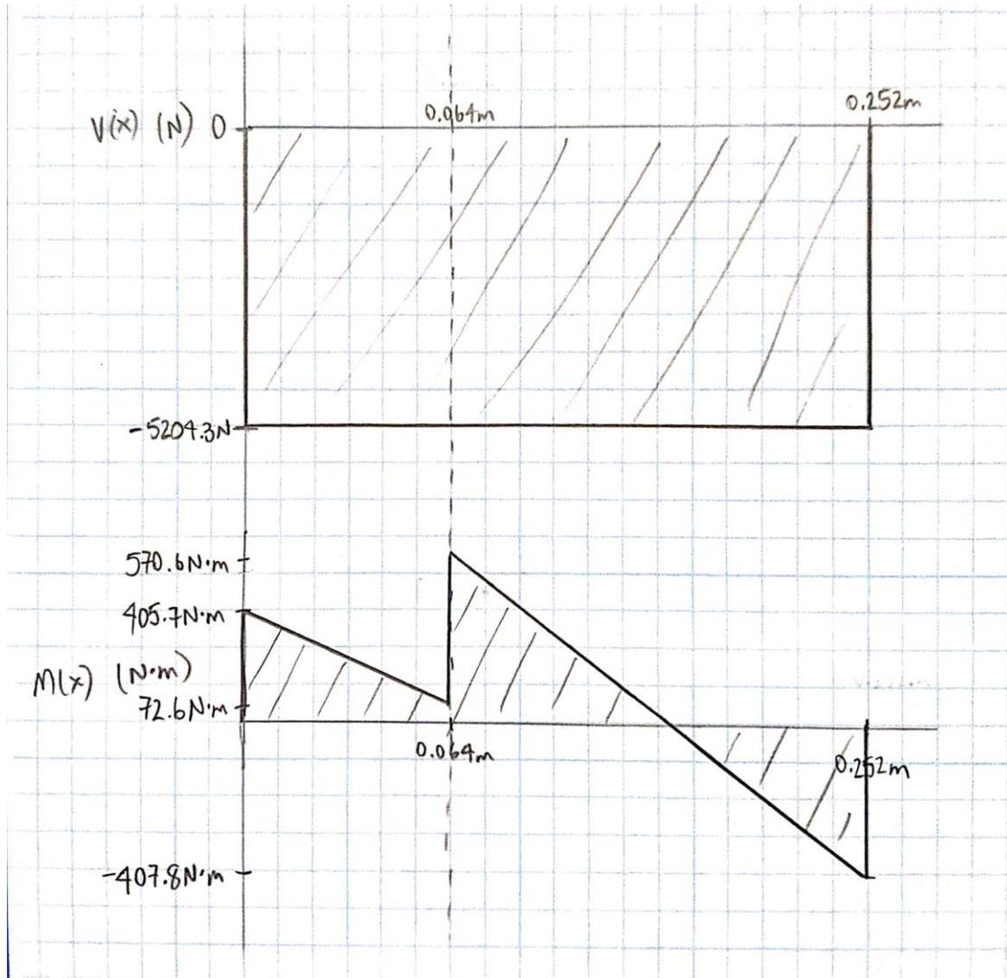
**Figure E35:** Shear force and bending moment diagram for calculated differential hanger web.
