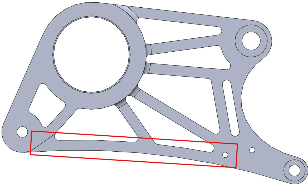
**Figure E34:** Left differential hanger highlighting single web being calculated for maximum stress.
