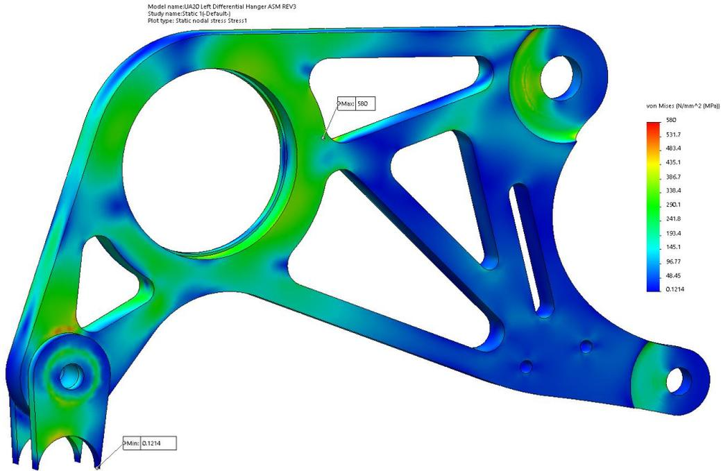
**Figure E15:** vonMies results for iteration 1 – view #1.
