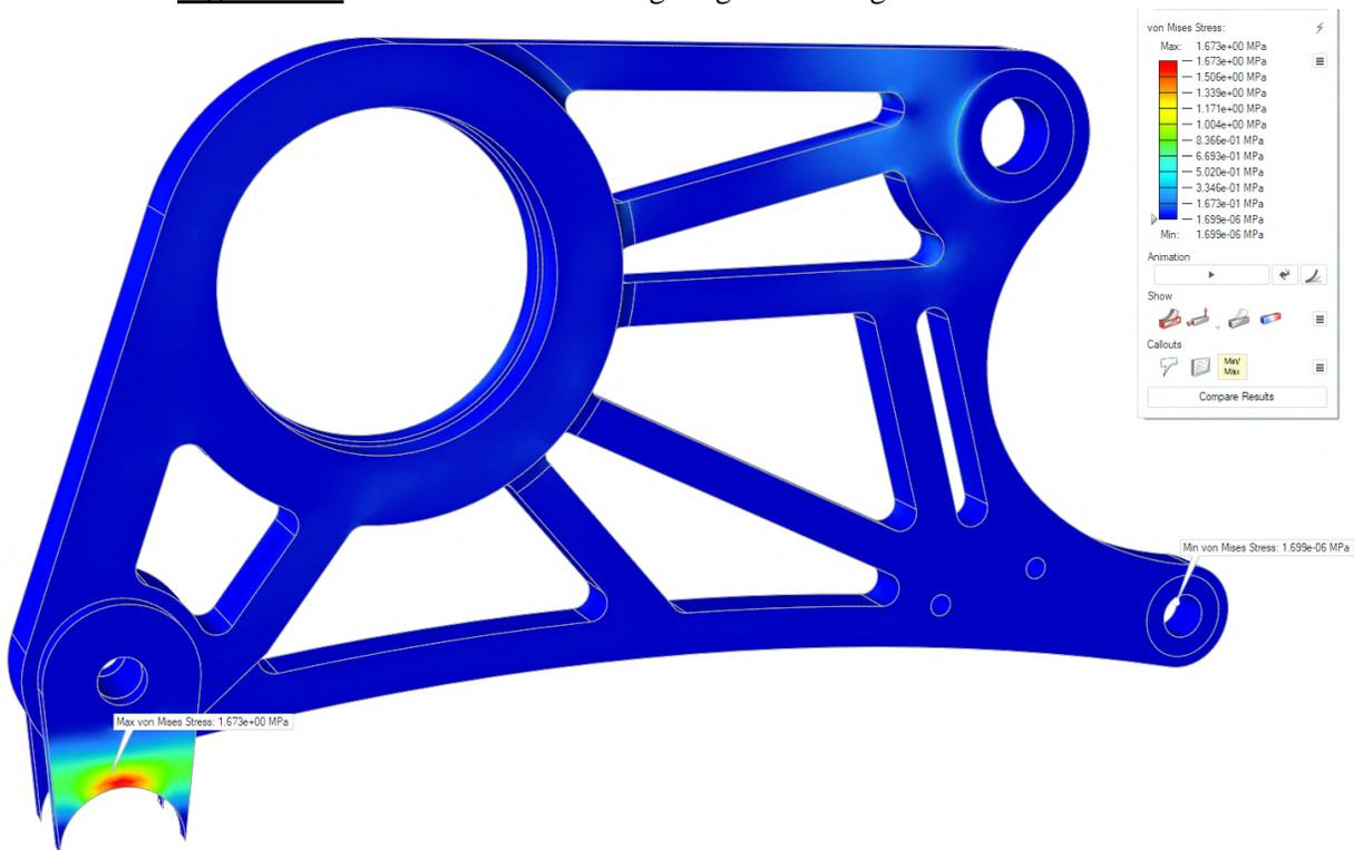
**Figure E33:** vonMises results for 2 g lateral engine mass acceleration.
