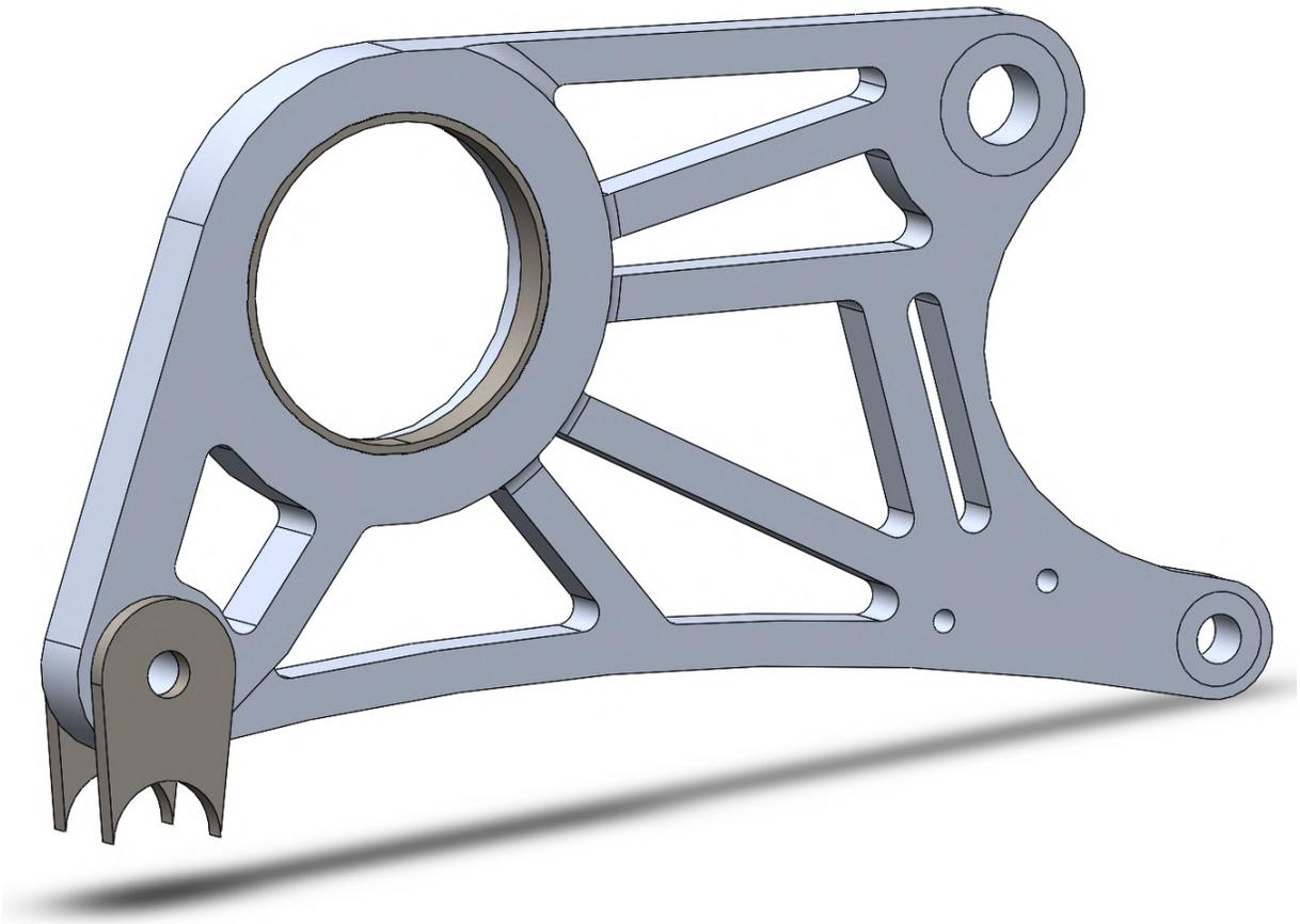
**Figure E26:** Inner bearing race added to final design static study.
