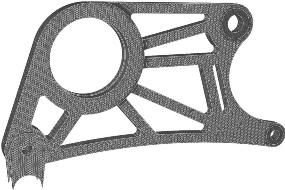
**Figure E31:** Altair Inspire 2019.3 mesh with average global element size of 1.5875 mm and a mesh control of element size 0.8 mm.
