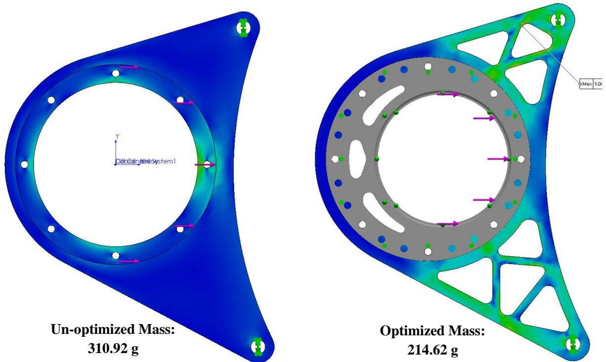
**Figure C3:** UA-19 differential hangers highlighting the weight saving results from topological optimization.
