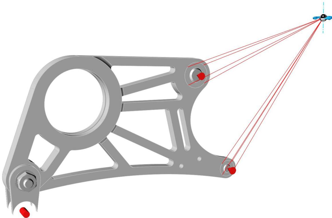
**Figure E30:** 2 g lateral engine mass acceleration applied to the differential hanger in Altair Inspire 2019.3
