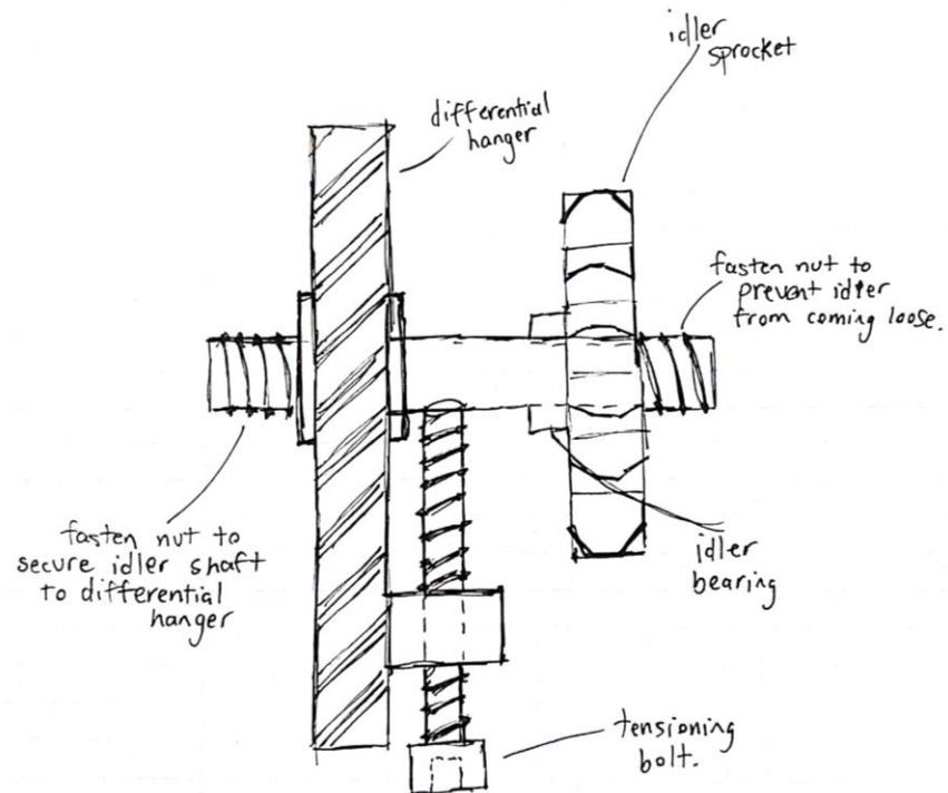
**Figure 8:** Hand drawn sketch of the UA-20 idler sprocket tensioning system.
