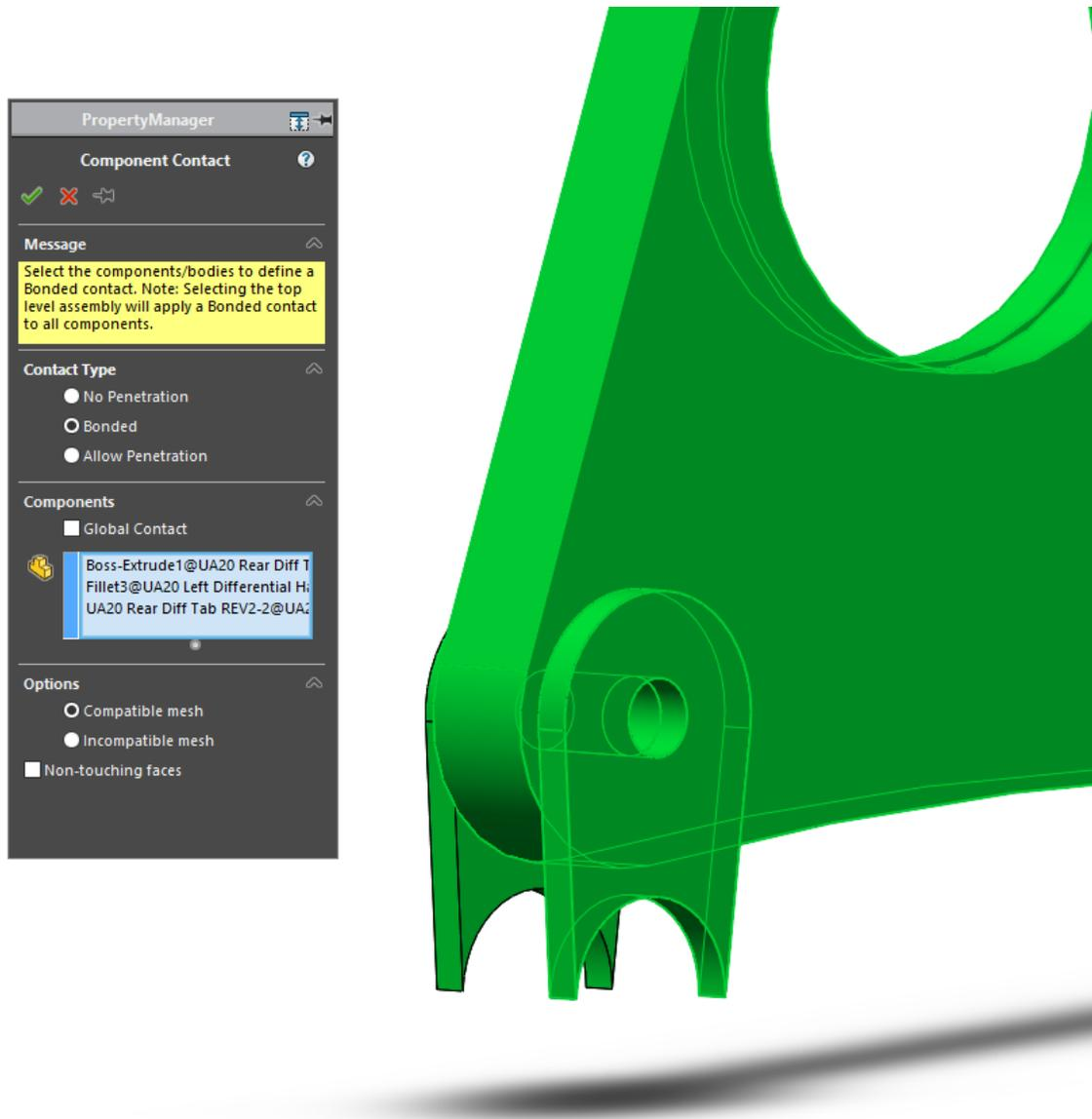
**Figure E2:** Component contact between differential hanger and tabs.
