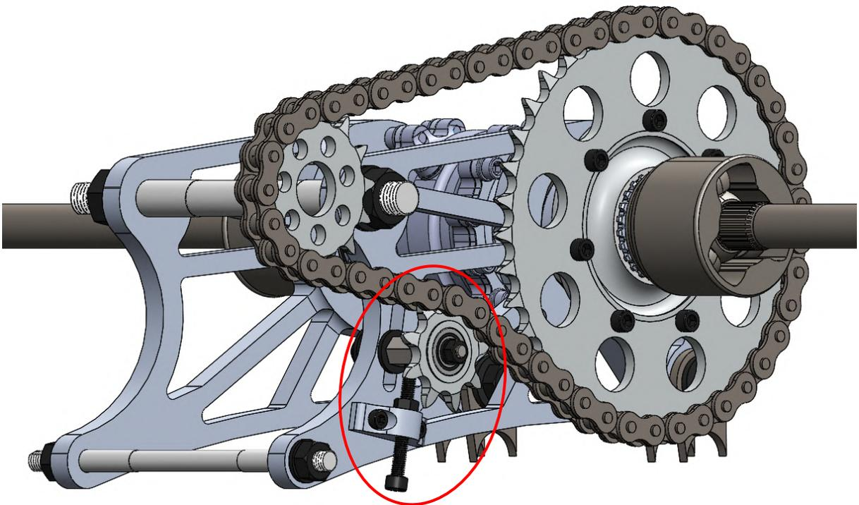
**Figure 12:** UA-20 idler sprocket assembly used to manually pre-tension the chain.
