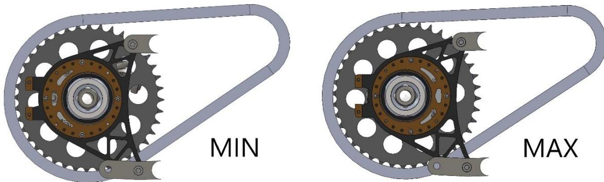
**Figure 4:** 3D CAD model cross sectional view of the drivetrain assembly highlighting the adjustability of the eccentric disk chain tensioner.
