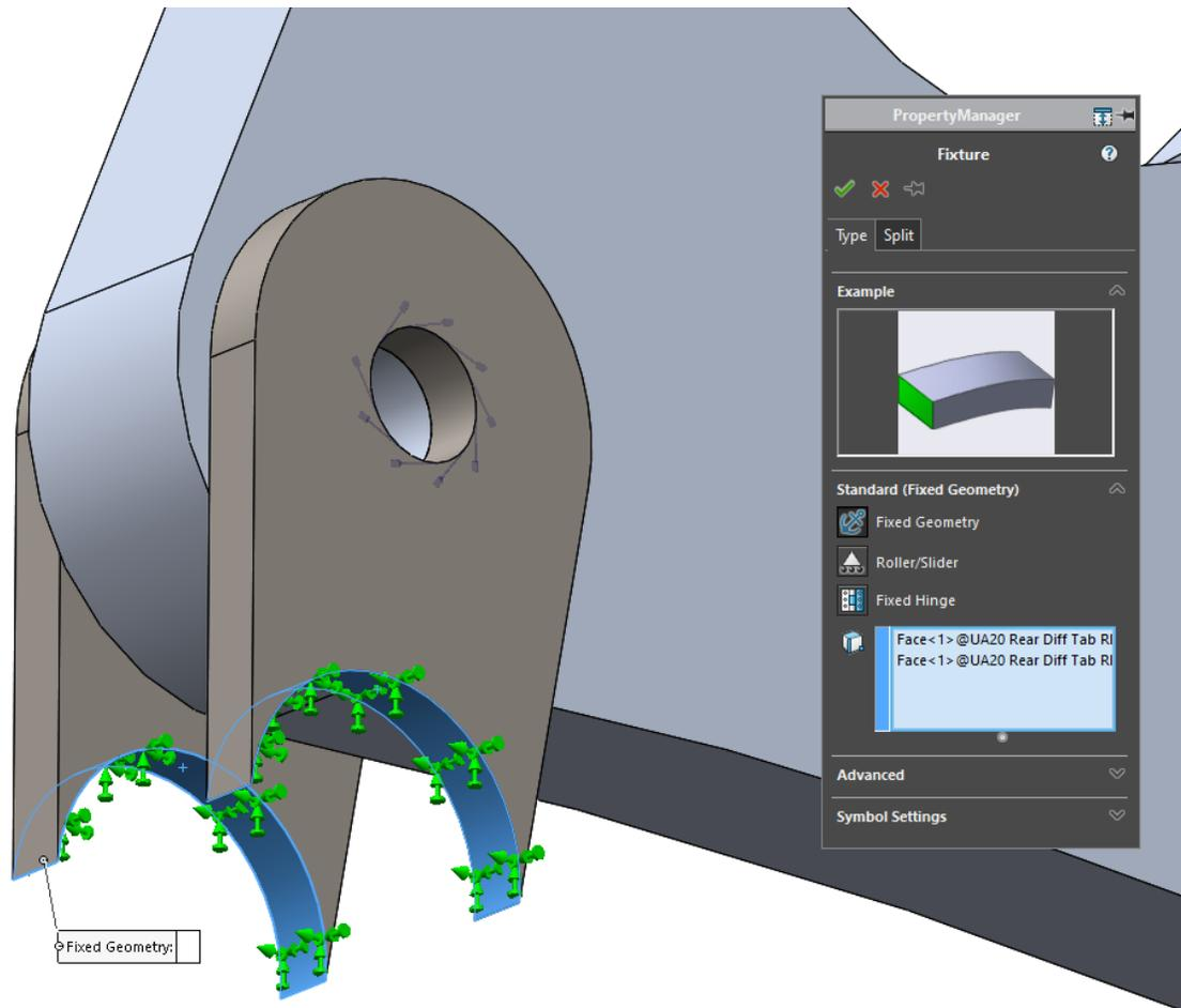
**Figure E4:** Fixed geometry mounting tabs.
