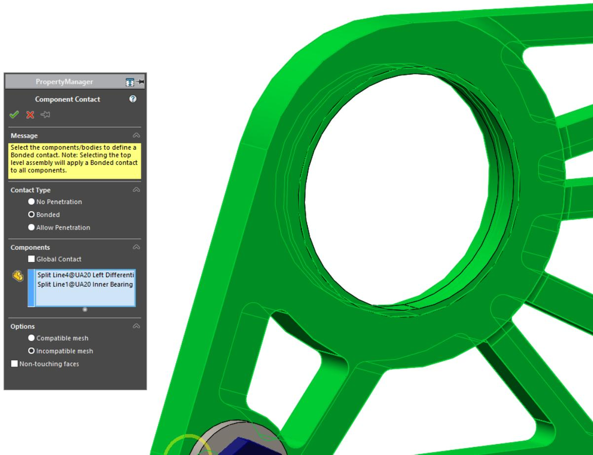
**Figure E27:** Bonded contact between inner bearing race and differential hanger.
