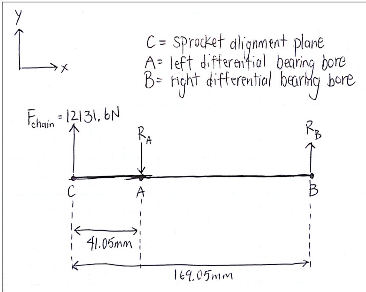
**Figure D8:** Free body diagram showing the maximum chain force and reaction forces at both differential hangers.
