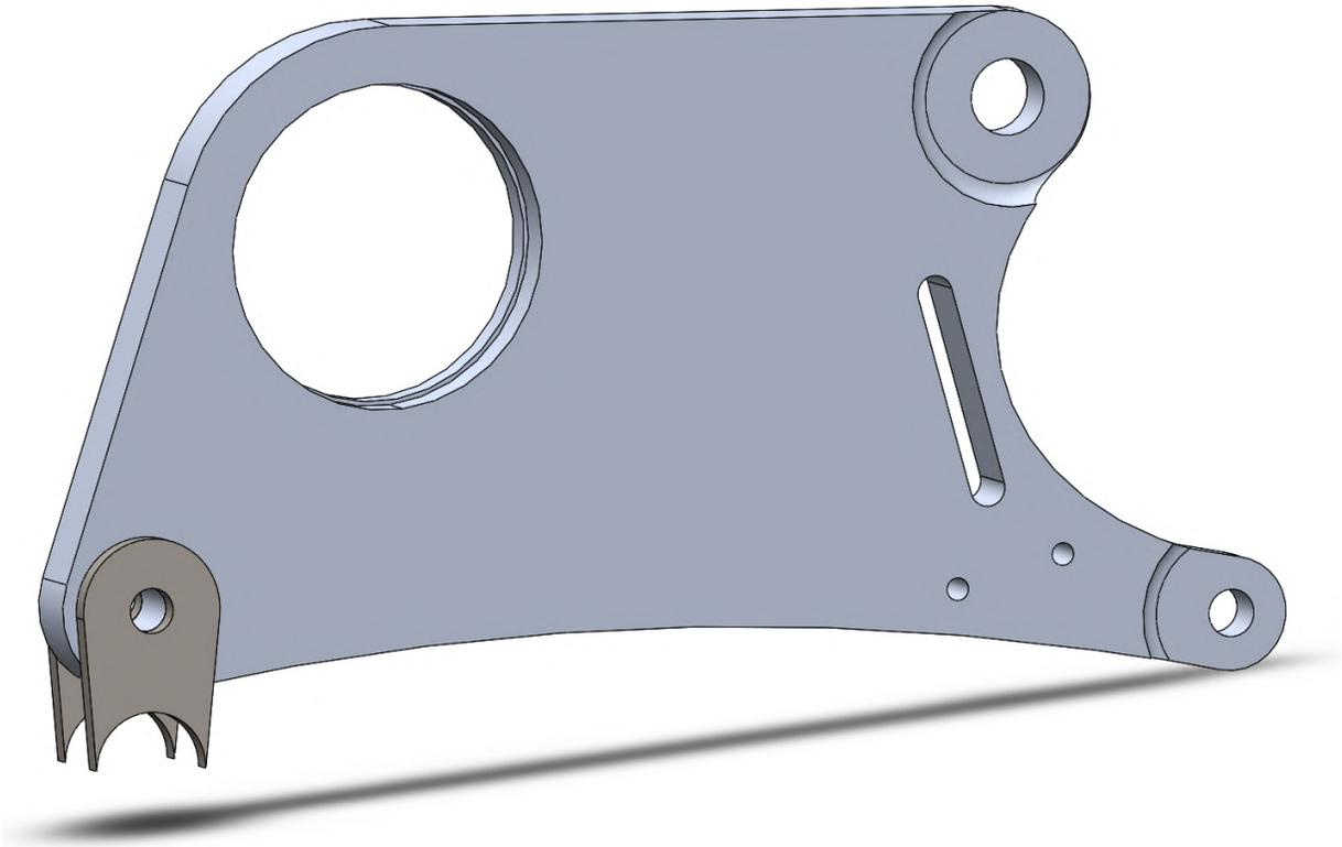
**Figure E1:** Baseline study assembly which includes rear mounting tabs.
