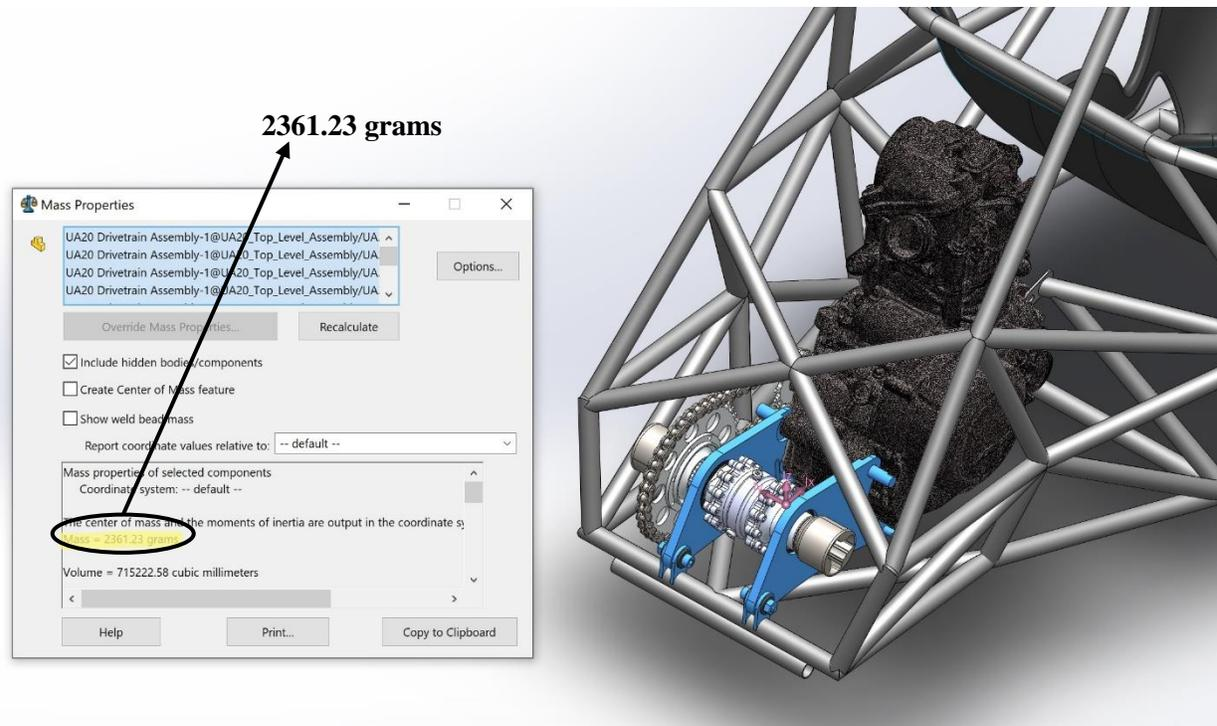
**Figure C2:** UA-20 drivetrain concept SolidWorks mass evaluation.
