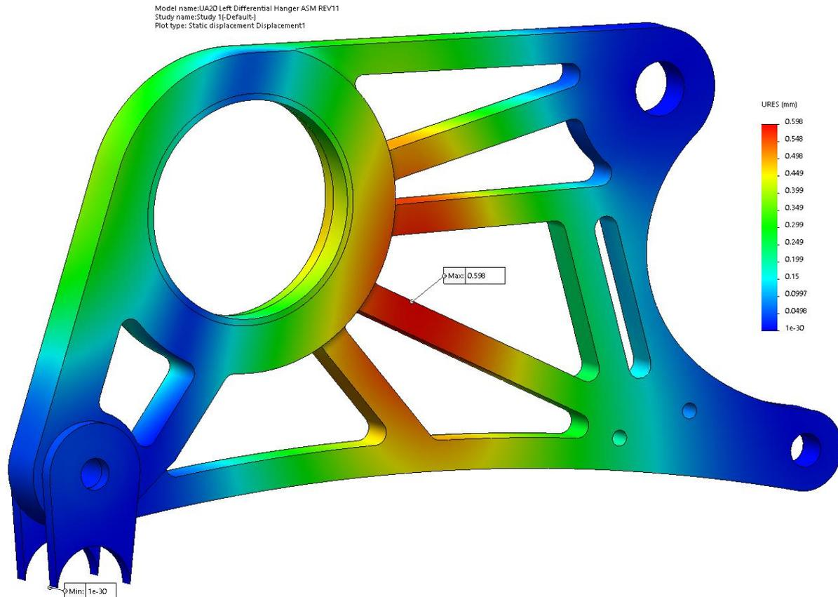
**Figure E28:** Final design with inner bearing race results showing maximum deflection of 0.598 mm.
