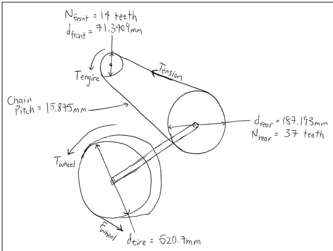
**Figure D2:** Free body diagram of chain, sprockets and wheel.
