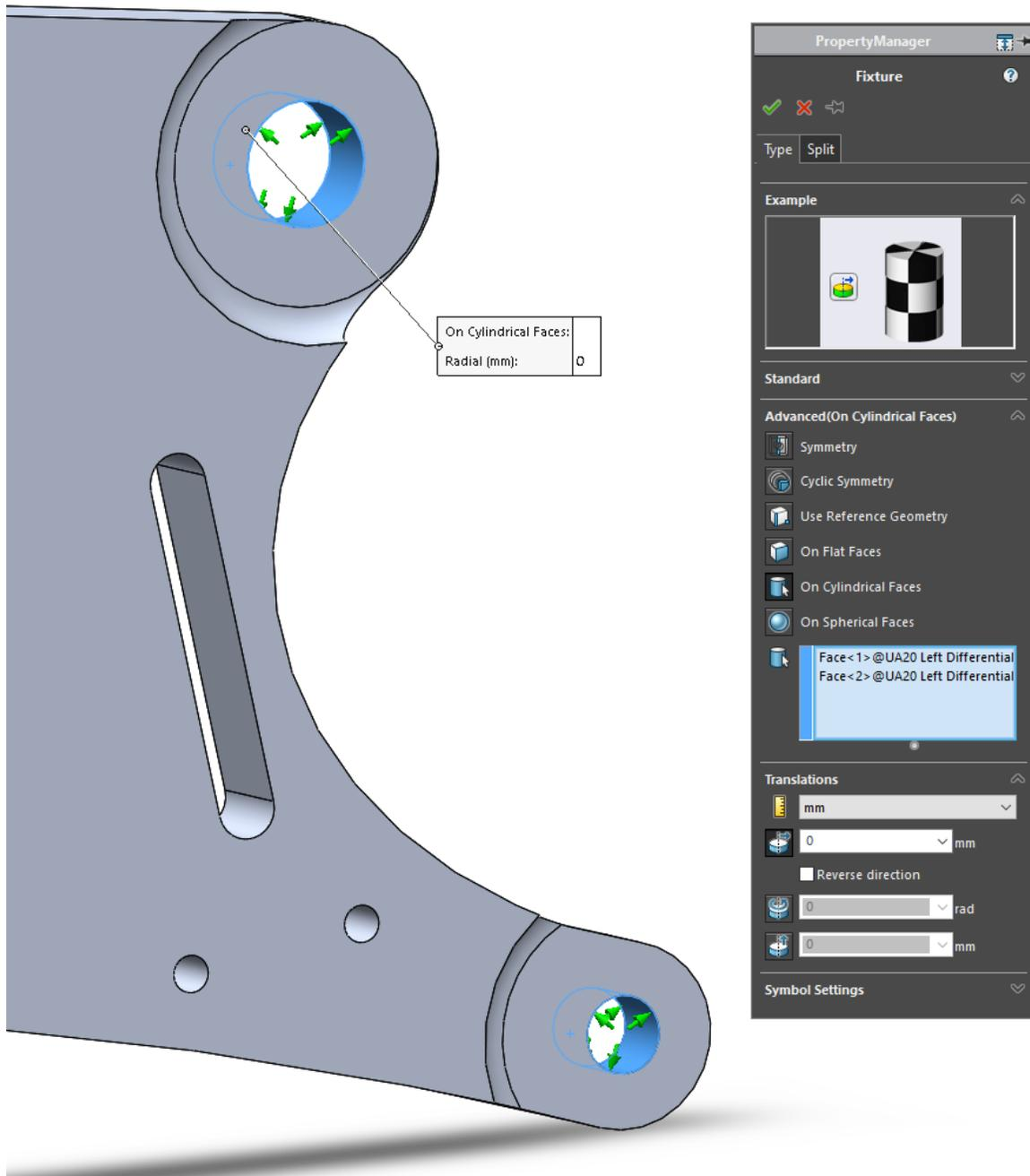
**Figure E5:** Advanced on cylindrical faces fixture to engine mount holes.
