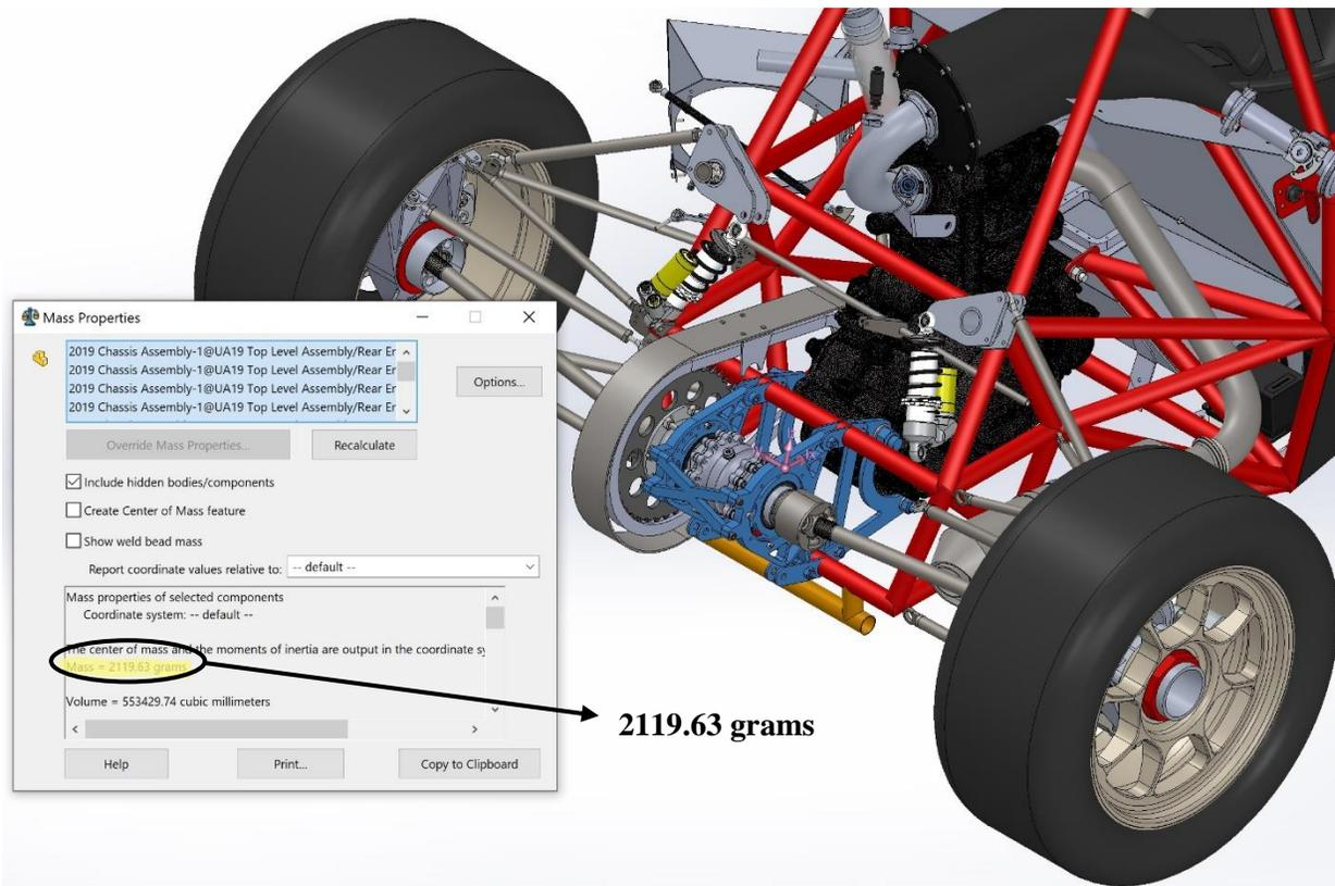
**Figure C1:** UA-19 drivetrain design SolidWorks mass evaluation.
