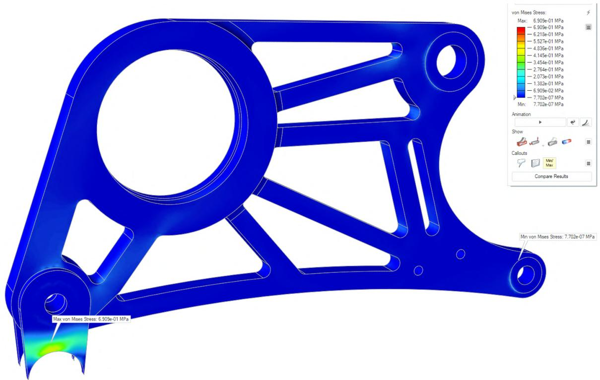
**Figure E32:** vonMises results for 2 g longitudinal engine mass acceleration.
