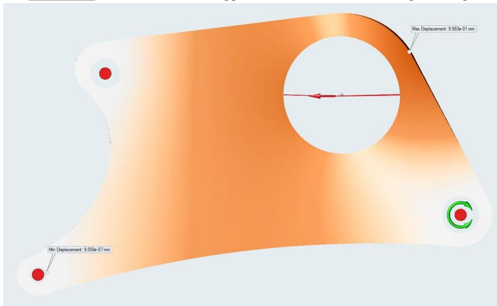
**Figure B5:** UA-20 concept deformation results. Maximum displacement of  $9.993 \cdot 10^{-1}$  mm.
