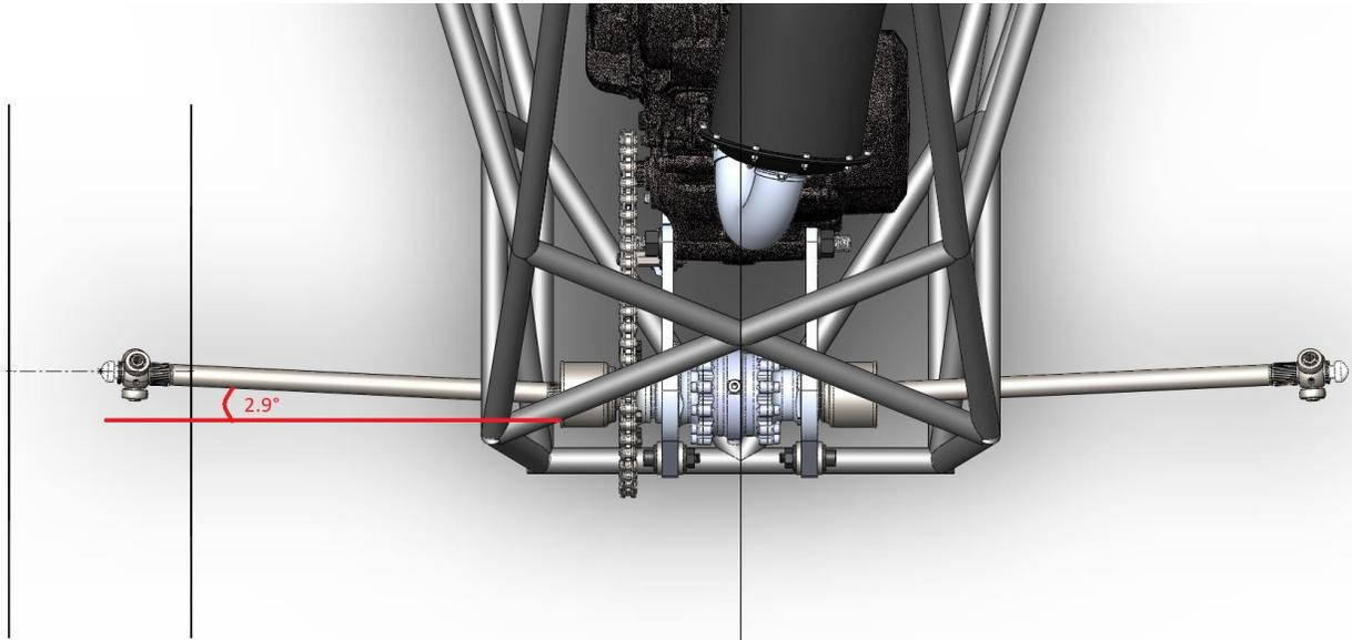
**Figure 11:** UA-20 driveshaft angles reduced to 2.9°.
