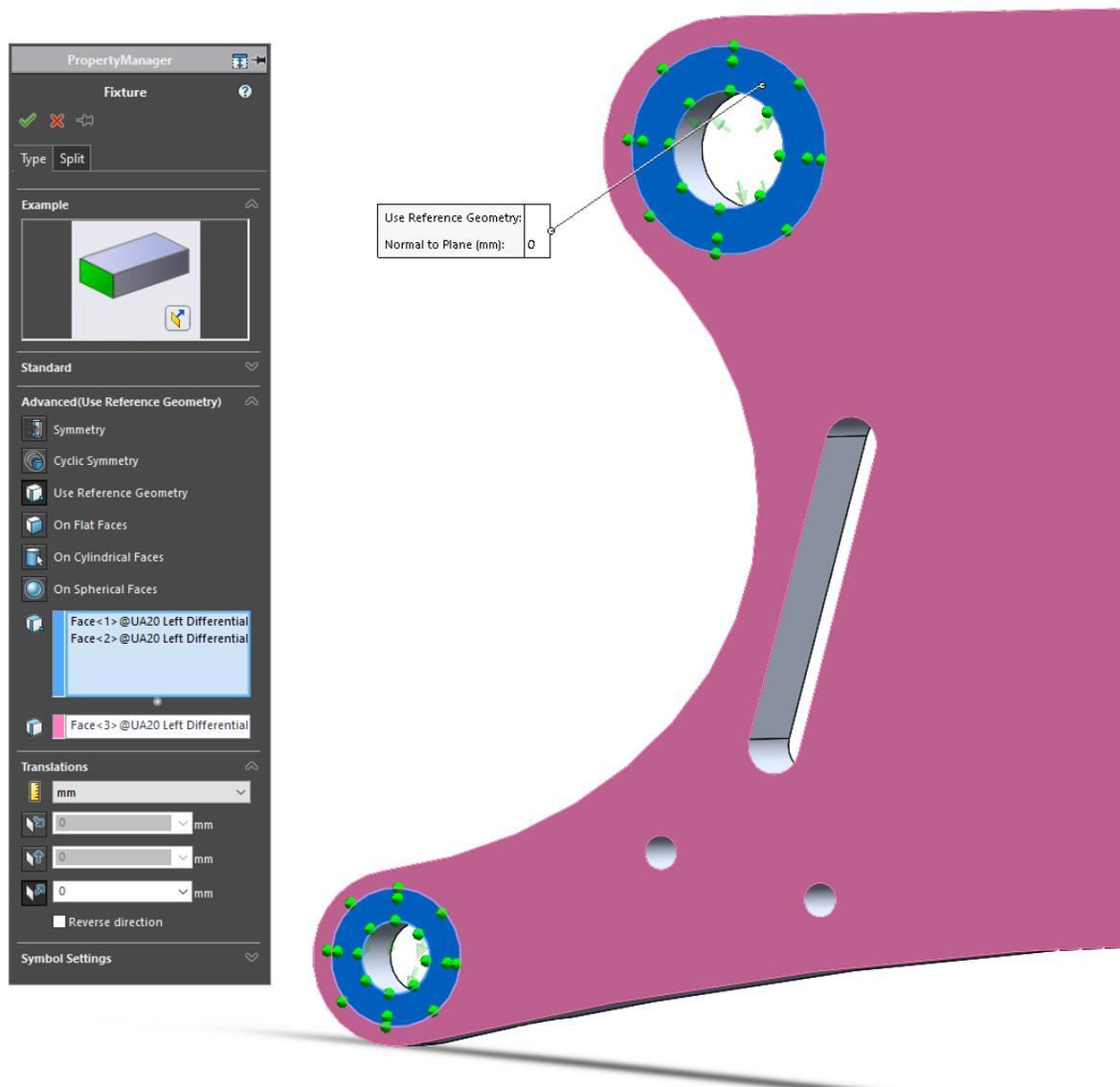
**Figure E6:** Advanced reference geometry fixture on washer split lines.
