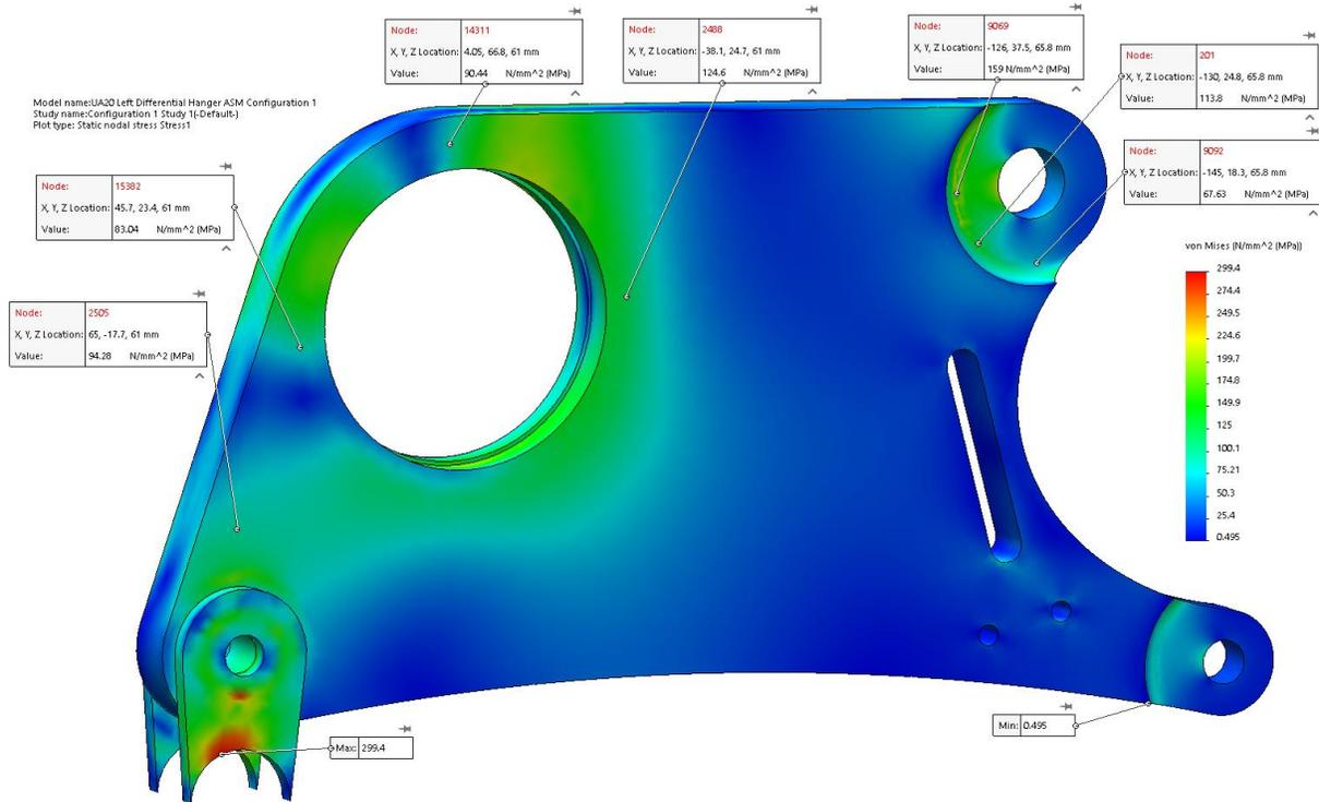
**Figure E12:** von Mises results for mesh 1 with probed sensor locations shown.
