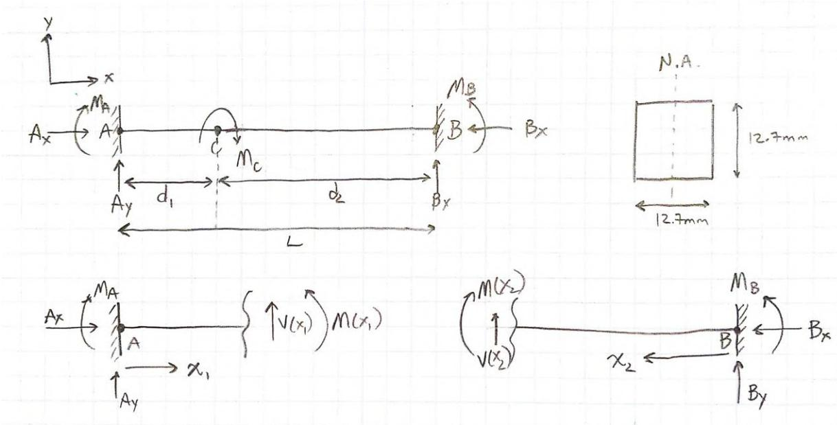
$M_C = 498 \text{ N} \cdot \text{m}$  (maximum moment caused by chain force)
