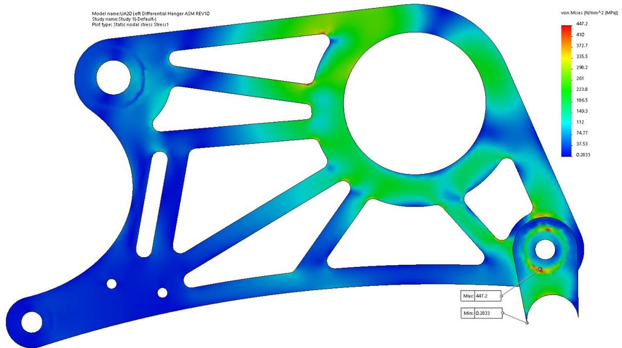
**Figure E21:** Final design von Mises results – view #3.
