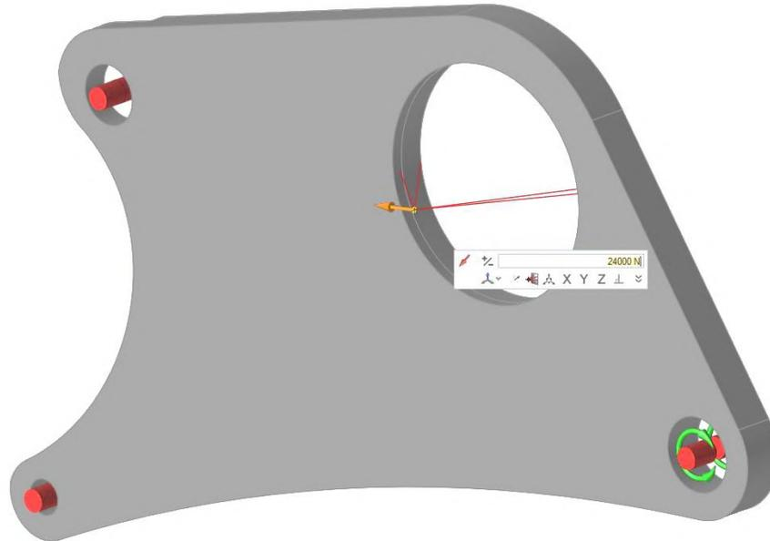
**Figure B4:** Constraints and load applied to UA-20 differential hanger concept.
