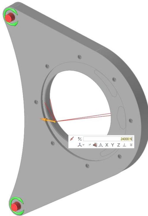
**Figure B2:** Constraints and load applied to UA-19 differential hanger design.
