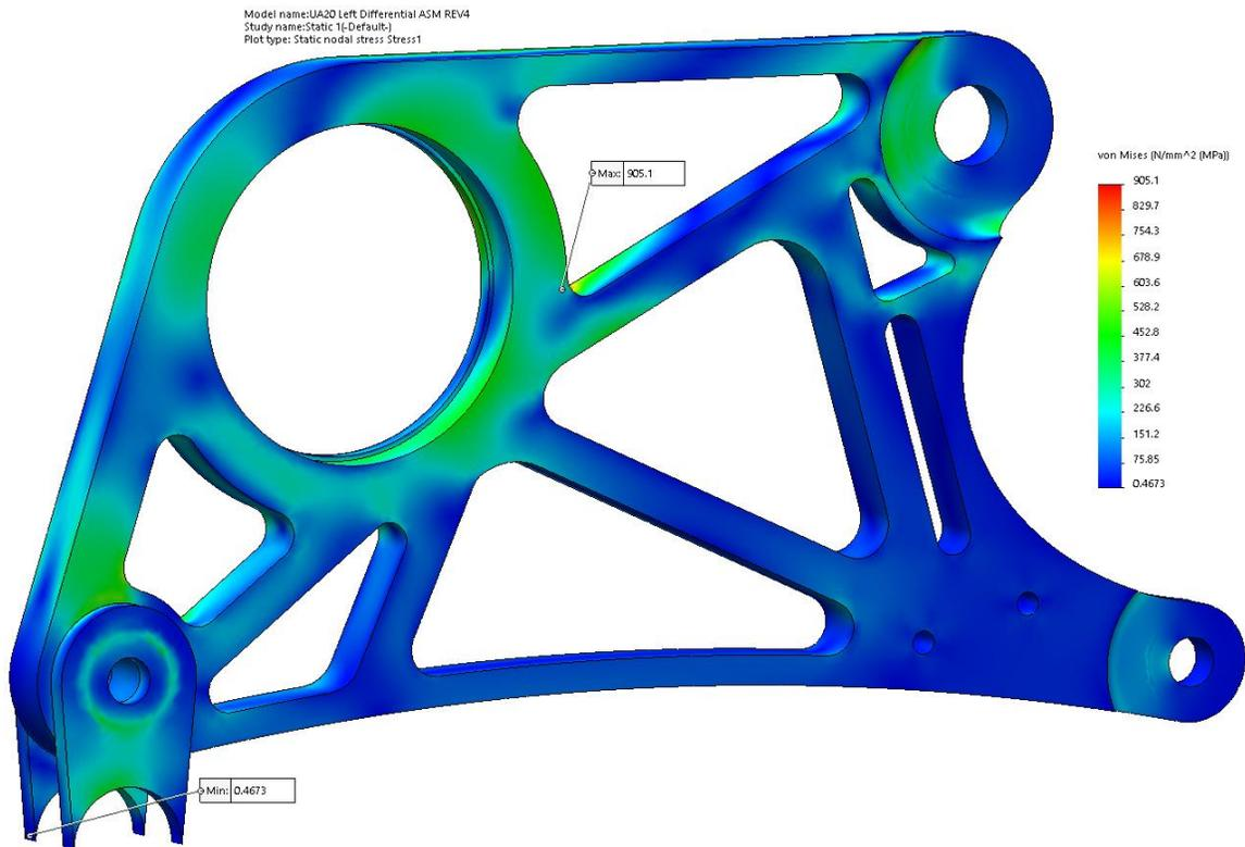
**Figure E17:** vonMises results for iteration 2 – view #1.
