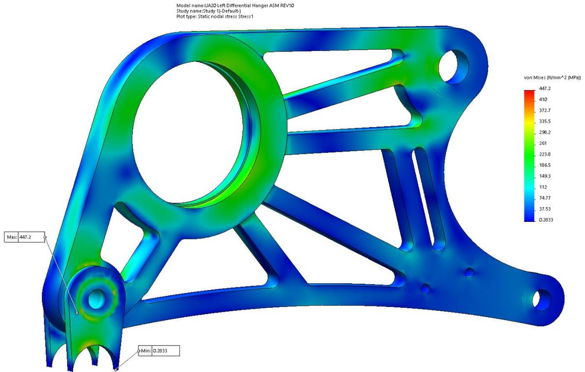
**Figure E19:** Final design von Mises results – view #1.
