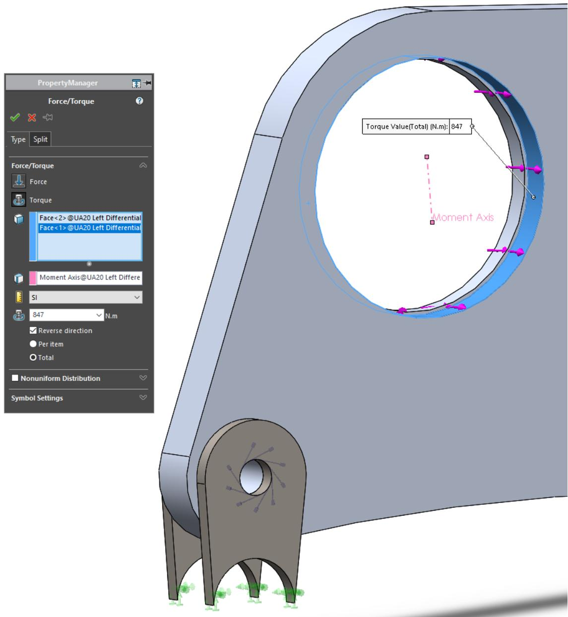
**Figure E9:** Torque applied to moment axis.
