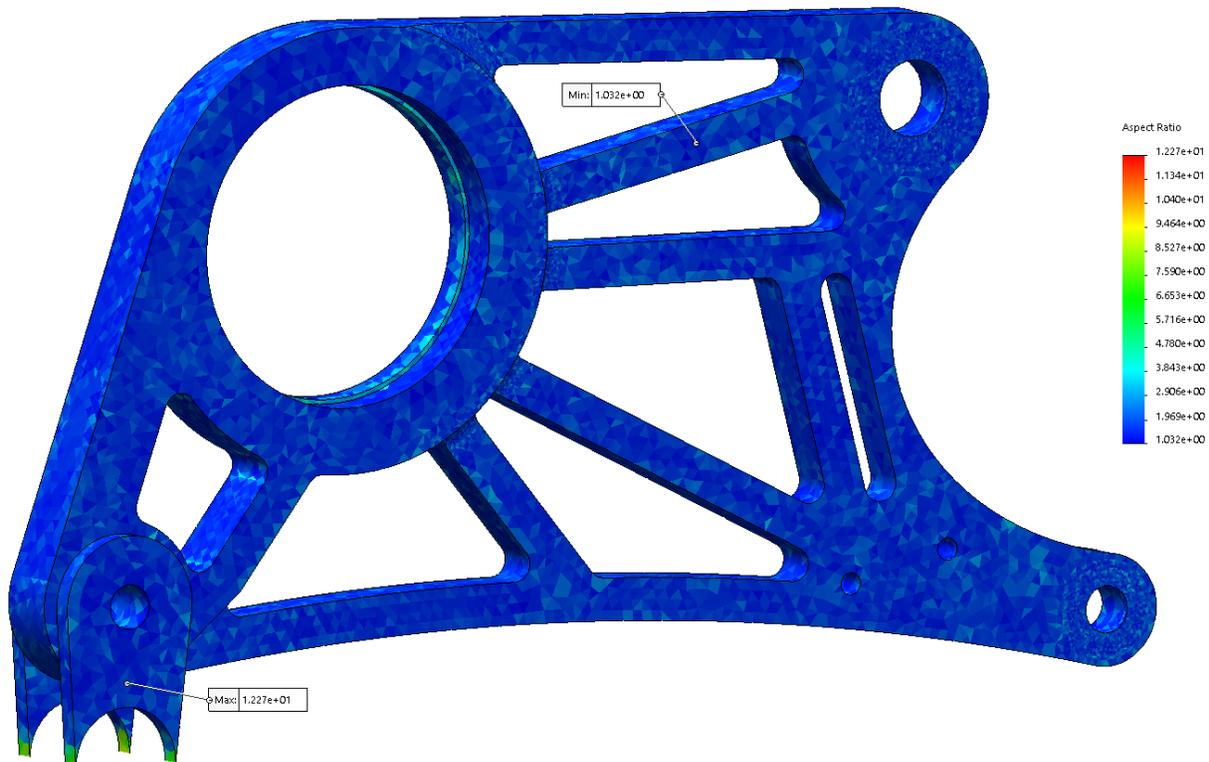
**Figure E23:** Aspect ratio mesh quality plot.
