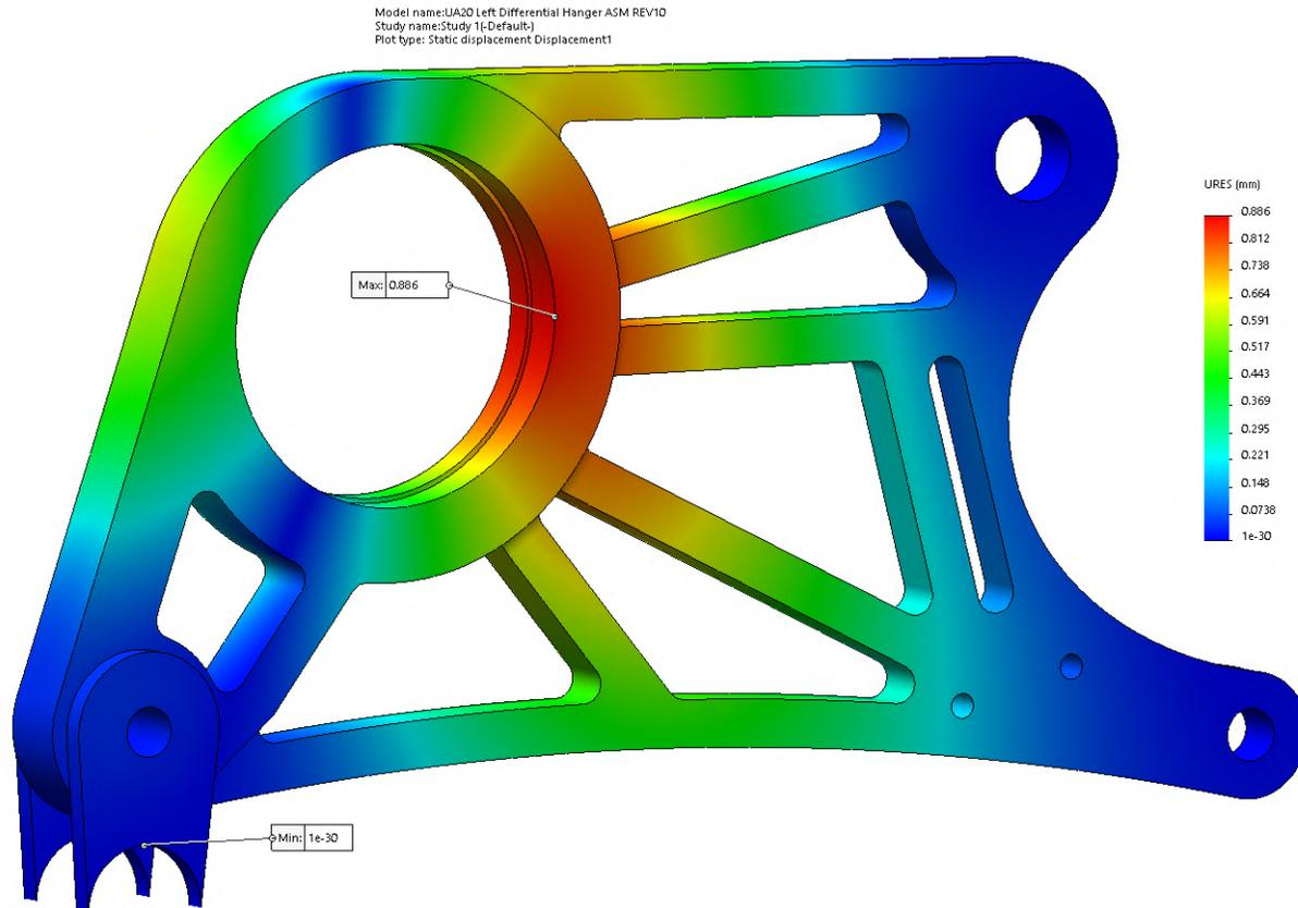
**Figure E24:** Final design displacement results showing maximum deflection of 0.886 mm.
