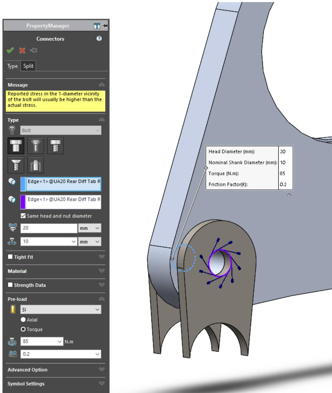
**Figure E3:** Nut and bolt connect through both mounting tabs.
