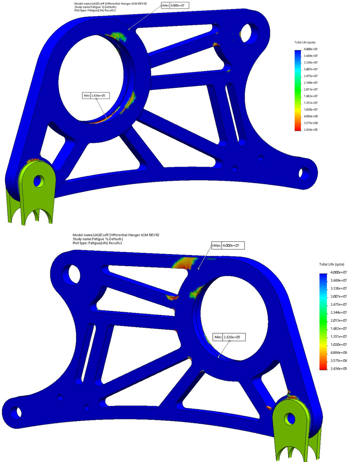
**Figure E25:** Fatigue study showing minimum number of cycles of 2.636e+05 before damage occurs.
