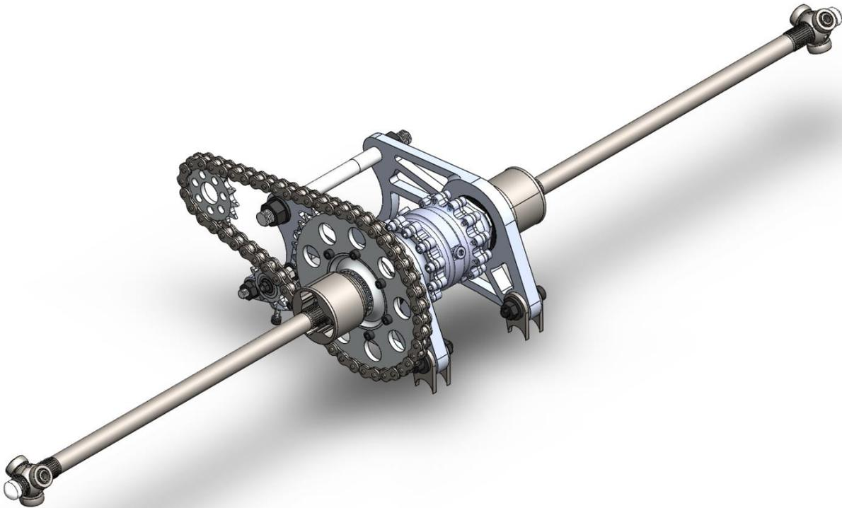
**Figure 10:** UA-20 final drivetrain assembly design.
