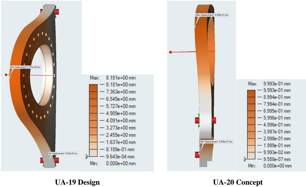
**Figure 6:** Displacement study performed in Altair Inspire 2019.3 comparing maximum deflection of UA-19 design and UA-20 concept. Both deformed states pictured above are exaggerated equally.
