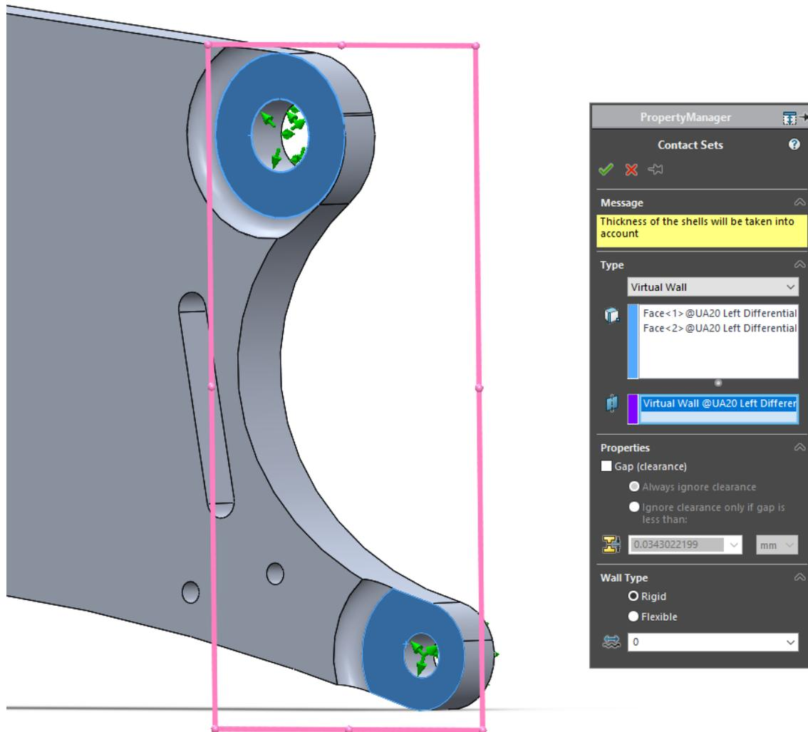
**Figure E7:** Virtual wall contact set applied to engine contact regions.
