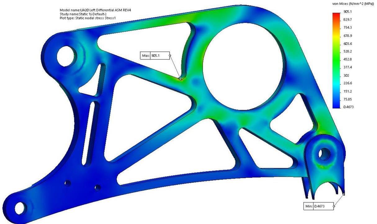
**Figure E18:** vonMises results for iteration 2 – view #2.
