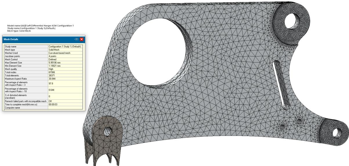
**Figure E10:** Mesh 1 with maximum element size of 5.95 mm throughout the differential hanger and a mesh control size of 1.2 mm throughout the engine mounting points.
