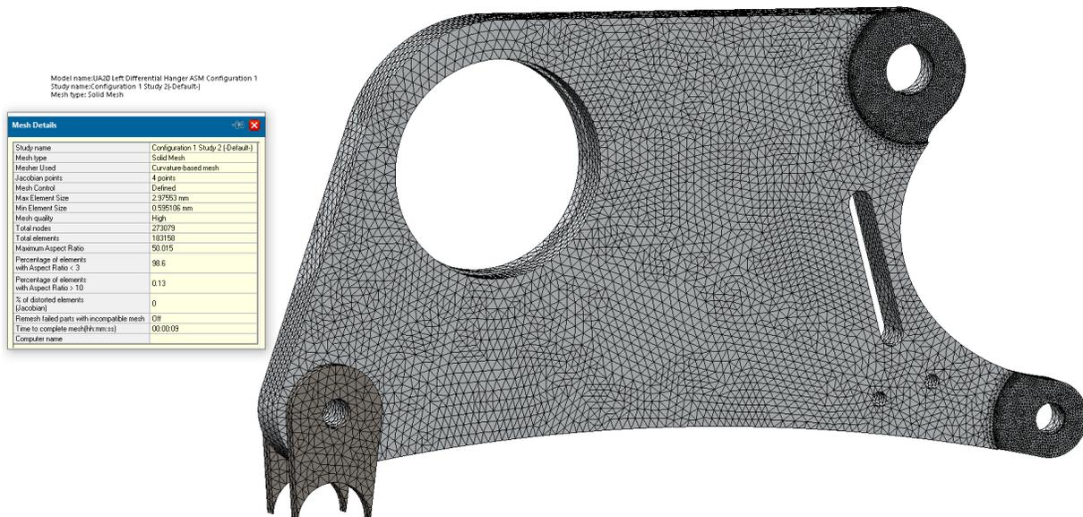
**Figure E11:** Mesh 2 with maximum element size of 2.97 mm throughout the differential hanger and a mesh control size of 0.8 mm throughout the engine mounting points.
