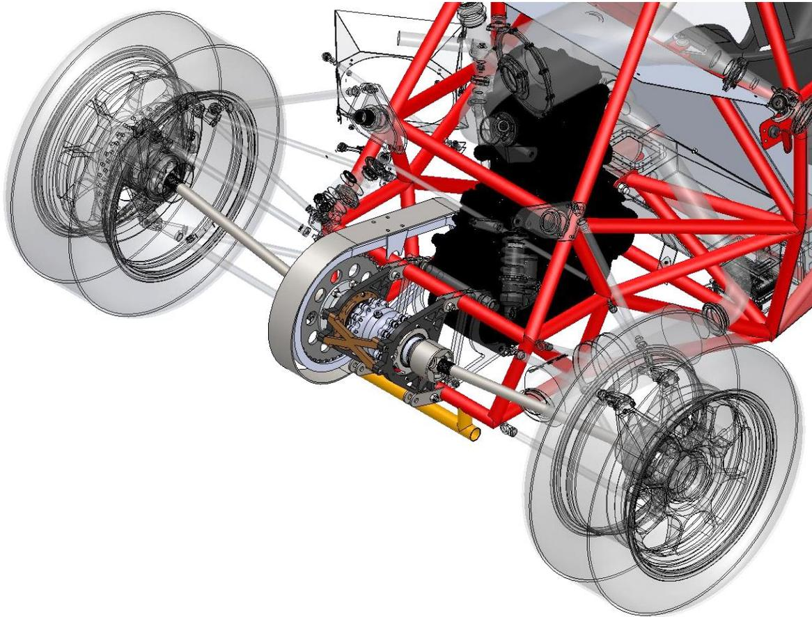
**Figure 1:** 3D CAD model isometric view of the UA-19 car highlighting externally mounted drivetrain system to the rear of the chassis.
