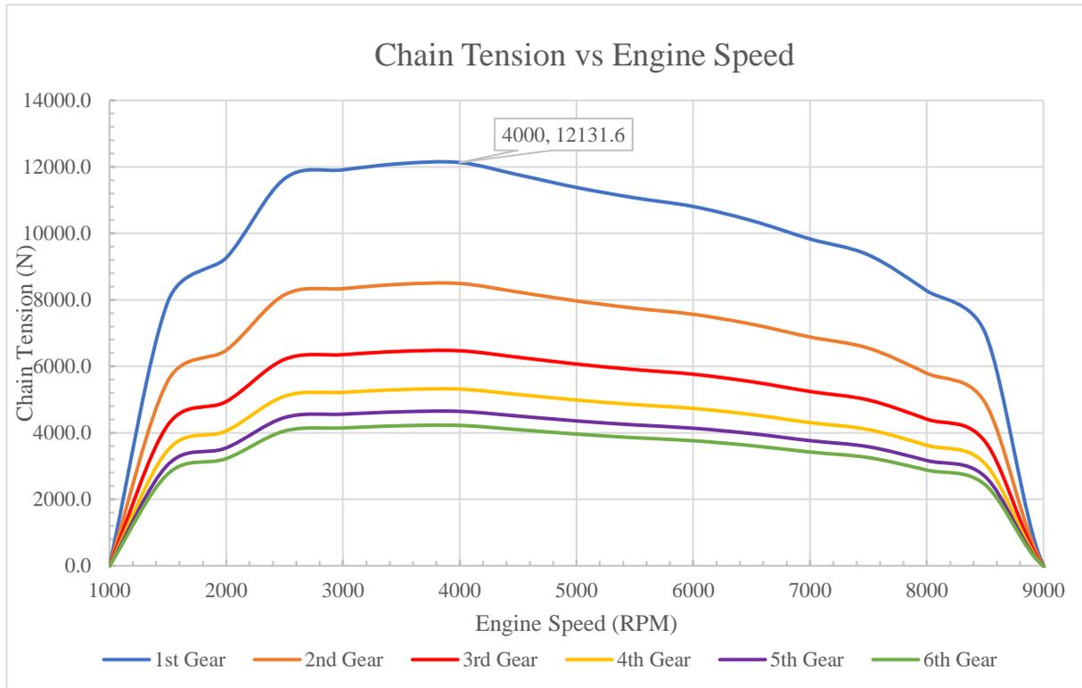
**Figure 13:** Chain tension (N) vs. Engine Speed (RPM) carried through KTM 690 6-speed transmission.
