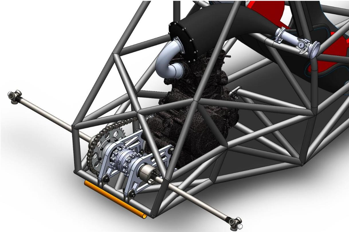
**Figure 9:** UA-20 final drivetrain assembly design packaged with the KTM 690 engine and chassis.
