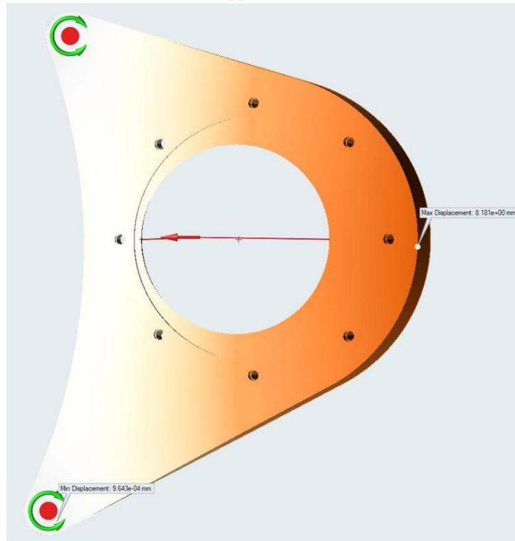
**Figure B3:** UA-19 design deformation results. Maximum displacement of  $8.181 \cdot 10^0$  mm.
