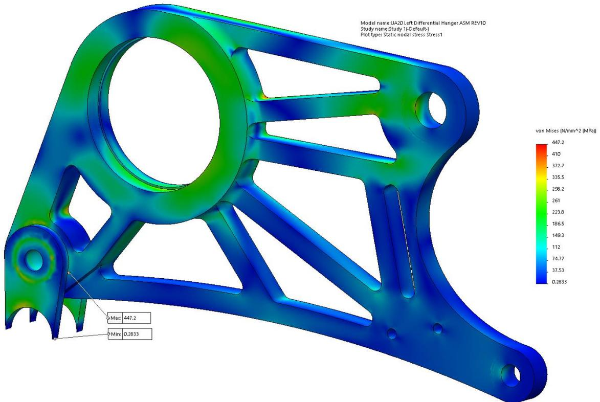
**Figure E20:** Final design von Mises results – view #2.
